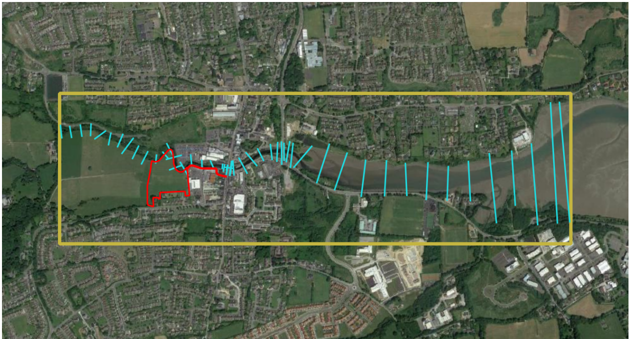
Figure 20: Cross-section location of river channel survey
